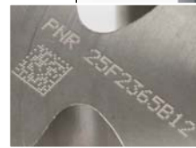
Marking DataMatrix™ codes in aeronautics subcontracting
