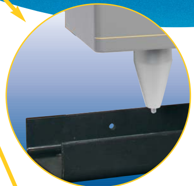
Marks on beams
